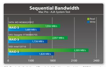
P.S : Due to the limitation of Thunderbolt 3 cables and hard drives, RAID 5 supports read speed up to 2,600MB/s and write speed up to 1,700 MB/s.
